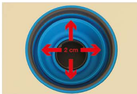
11. Maximum deviation: 4cm (plus/minus 2cm from the center)
