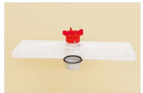
12. Insert the waste valve and screw it together with the counternut. The gasket has to be tight on the bottom of the tray
